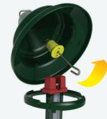
**2 Disconnect and remove the seed tube
